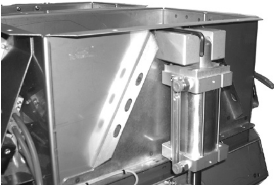
Figure 9-10: Adjust the space between the clevis block and the bucket lip
