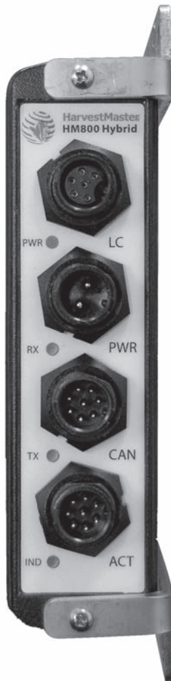
Figure 4-3: Side view of BDS Hybrid showing connectors and labels.
