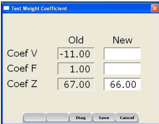
Figure 3-30: The new Coefficient Z value in this screen differs from the old value by -1.00
