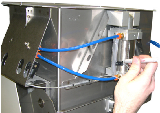
Figure 9-12: Use a marker to make the top edge of the limit switch
