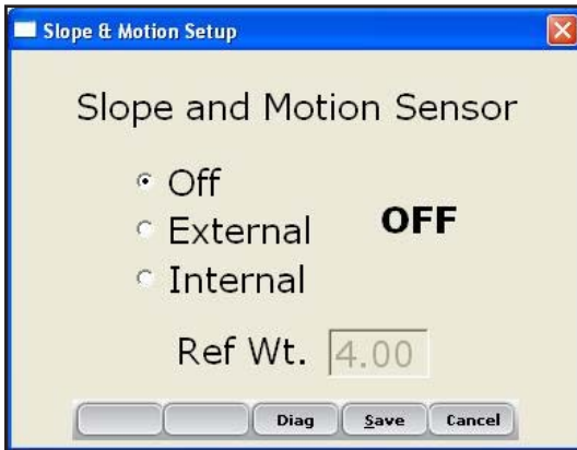
Figure 3-13: Slope and Motion Setup screen with the Slope and Motion Sensor turned off
