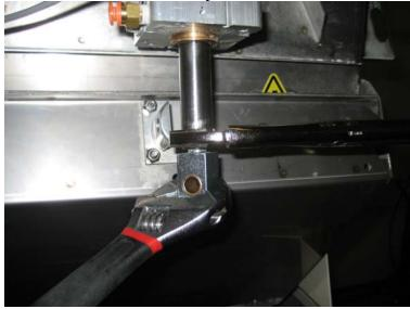
Place the 22438 Twin Bucket Cylinder Stop Collar over the cylinder as shown. It may have a tight fit but if aligned it
