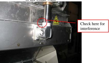
Re-attach the lower air line as shown. Repeat the same procedure on the cylinder on the other side.
