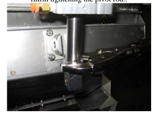
Remove the vise grips and re-insert the clevis pin and e-clip as shown. Check the door motion to be sure there are no interferences or problems, especially with the flange of the bucket. If interference in found here, the collar must be ground down on that side to allow the bucket to close completely. Grind more than half way through the thickness of the collar wall.
