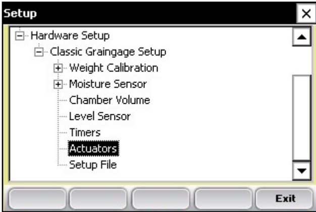
Figure 3-21: Double-tap Actuators from the Setup menu to access the Actuator Setup screen
