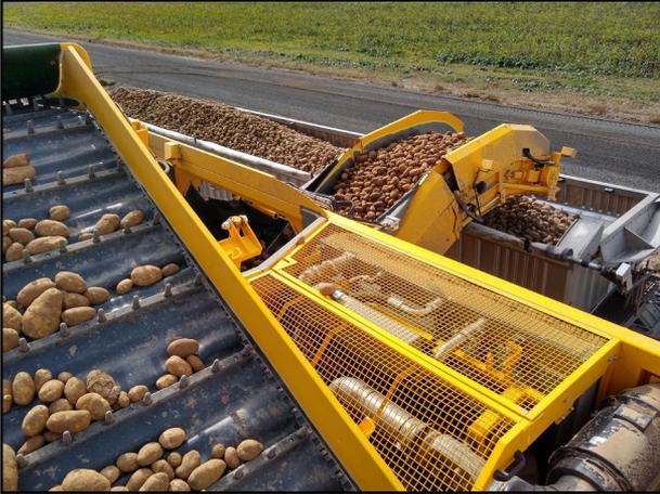
During harvest, the Casma system creates a yield map of your fields. It does this by simultaneously tracking belt speed, crop weight, and harvester movement. All this data is then sent to [mycasma.com](http://mycasma.com) and the cab of the harvester in the form of immediately actionable yield data, truck load weights, and harvester logistics (location, run time, idle time, total tonnage harvested by date, etc.).
