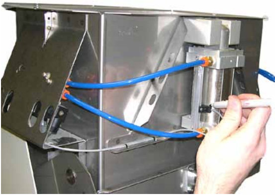
Figure 9-12: Use a marker to mark the top edge of the limit switch
