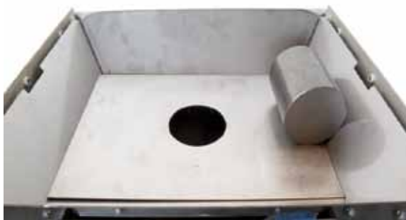
Figure 3-5: Place the weight on the right side of the weigh bucket
