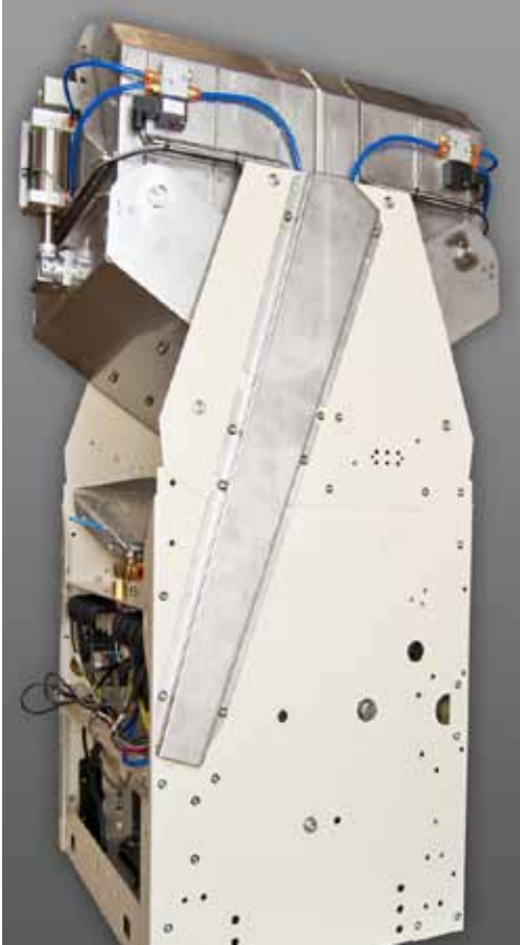
Figure D-5: Cable guard installed on HCGG
