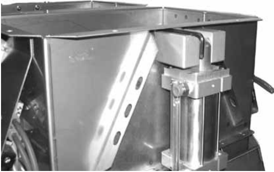
Figure 9-10: Adjust the space between the clevis block and the bucket lip
