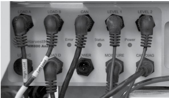
**Figure 4-6: Analog module showing CAN Terminator**
