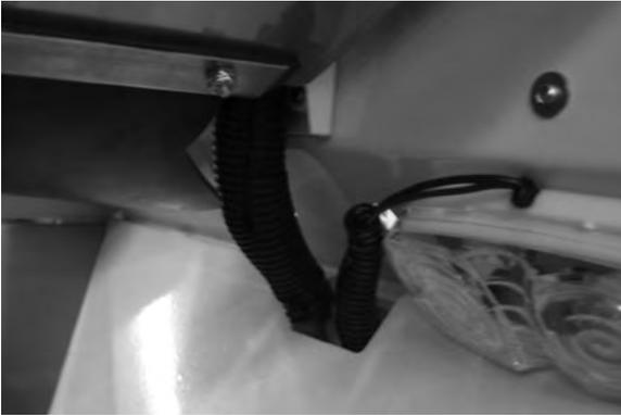
***Figure D-7: Cables coming down from top to the base of the HCGG***
