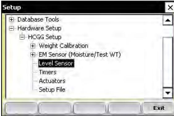
**Figure 7-14: Double tap Level Sensor from the Setup menu to access the Level Detect screen**
