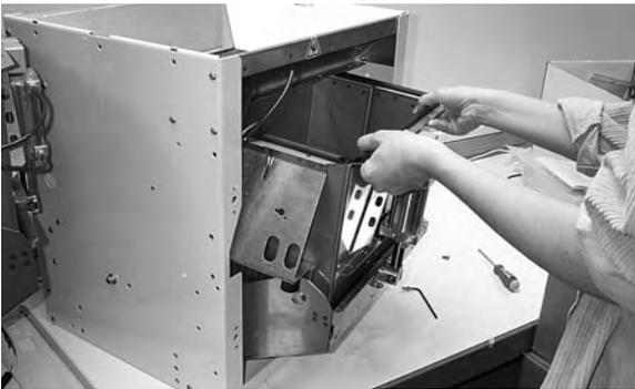
***Figure 9-17: Removing the weigh bucket***
