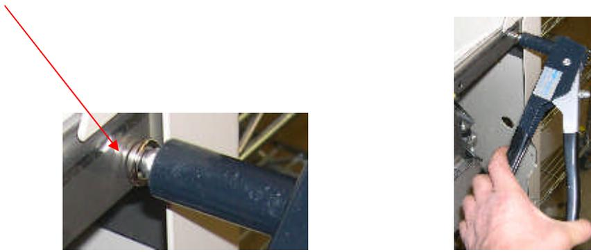
6. Check to make sure the button snap socket is secure.
