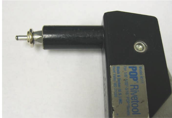
3. Insert the end of the pop rivet into one of the seven holes shown on the next page.
