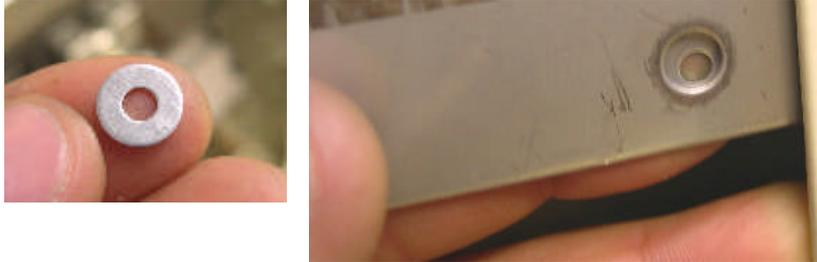
5. Make sure the button snap socket is flush with the surface, as shown in the picture on the left. Squeeze the tool and pop the rivet.
