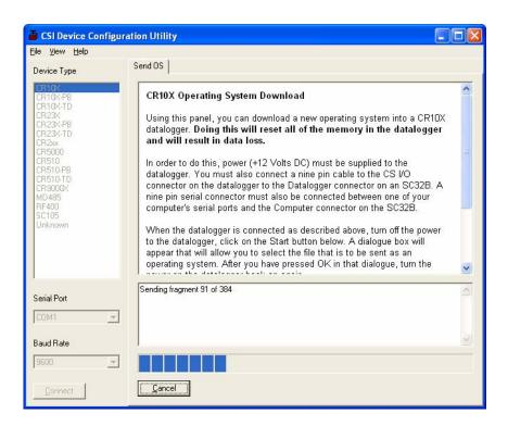
When the operating system has been sent to the device, a message dialog will appear similar to the one shown below:
