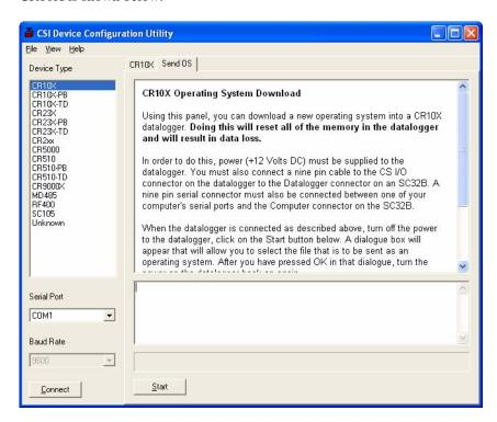
The text at right describes any interface devices or cabling required to connect the PC to the device. Screens for other devices vary only in the text on the right side. This screen differs from other screens that are available in DevConfig in that it can be accessed from either a connected and disconnected state.
