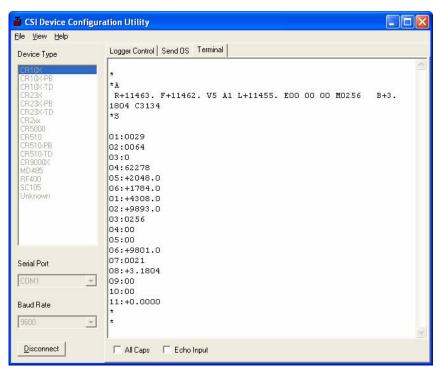
The default for the Terminal tab is to only show characters that are returned from the device. However, if the **Echo Input** check box is enabled, the screen will also display the characters actually typed by the user.
