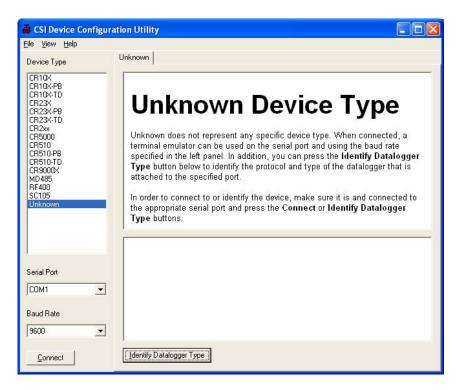
Clicking **Connect** puts DevConfig into Terminal emulation mode on the Serial Port and at the Baud Rate selected.
