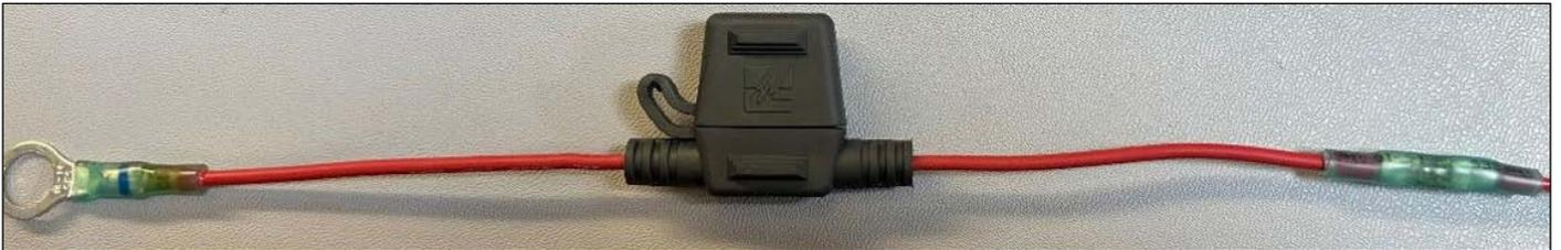
11. Connect the ring terminal to the battery.
