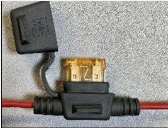
10. Place the ATC fuse (20 A) in the fuse holder and close the cap.
