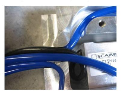
3. Insert screws through the bottom of the Load Cell Mount Bracket into the load cell. Leave screws snug so the load cell can be slid back and forth.
