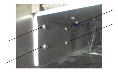
4. Remove the entire BDS assembly from the bucket, being careful not to damage the air hoses or load cell cable as you remove them from the hole in the side of the bucket. Clean out the button head screws on all locations of the BDS and use a high quality Allen wrench. We recommend replacing the four button head screws with ½ -20 by ¾ Socket Head Cap stainless steel screws (p/n 22743).
