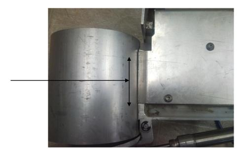
10. Install the BDS Sensor back in the bucket, making sure not to pinch or cut any hoses or wires as you fish them through the hole. Make sure to use the new ¼ -20 by ¾ Socket Head Cap stainless steel screws (p/n 22743) to bolt the sensor back in. Also make sure the sensor is squarely installed to the wall by sliding an Allen wrench or other object down the crack
