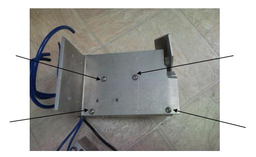
10. Flip assembly body upside down so striker arm is on the bottom.
