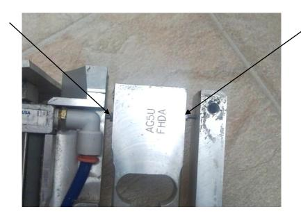
9. Check for final clearances on cup before reinstalling BDS sensor into bucket. You should be able to slide a business card between the thin plate and the cup and not have any binding issues.
