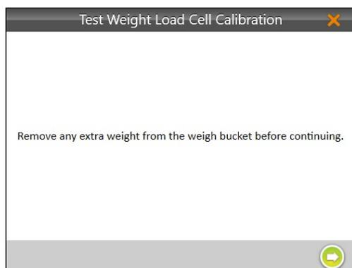
13. Check for and remove any extra weight from the weigh bucket.
