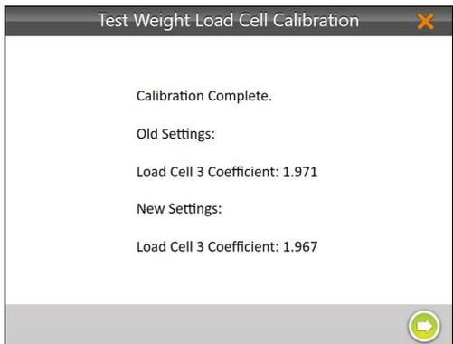
16. Mirus displays the old and new load cell coefficients.
