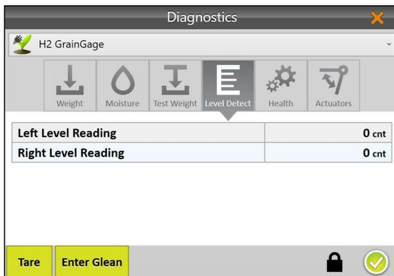
On the Level Detect Diagnostics screen, Mirus displays the status of the Level Detect Sensors. They should be at zero count when the hoppers are empty.
