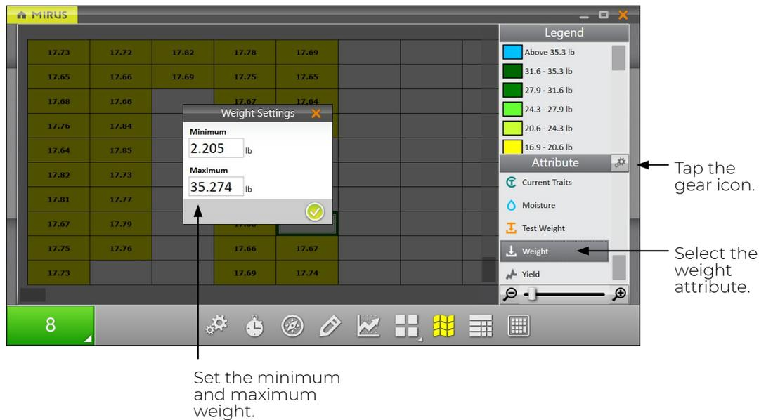
This setting adjusts the maximum weight on the Real Time Weight display, which allows you to track how full the GrainGage is getting with each plot. This is important to monitor so the GrainGage doesn't overflow.
