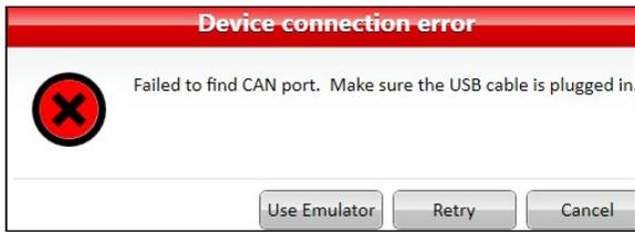
If Mirus is unable to detect the H2 GrainGage, the software may display a device connection error.
