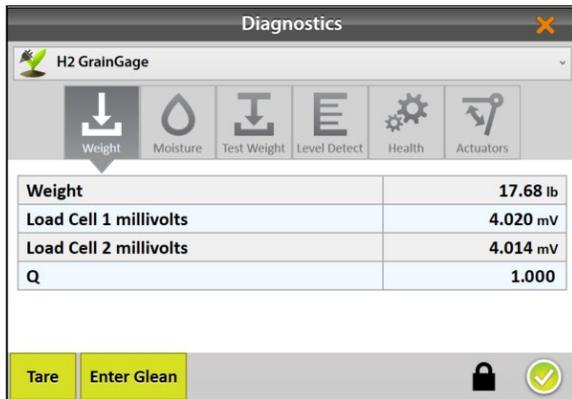
1. After calibrating the weigh bucket, tap the gear icon
