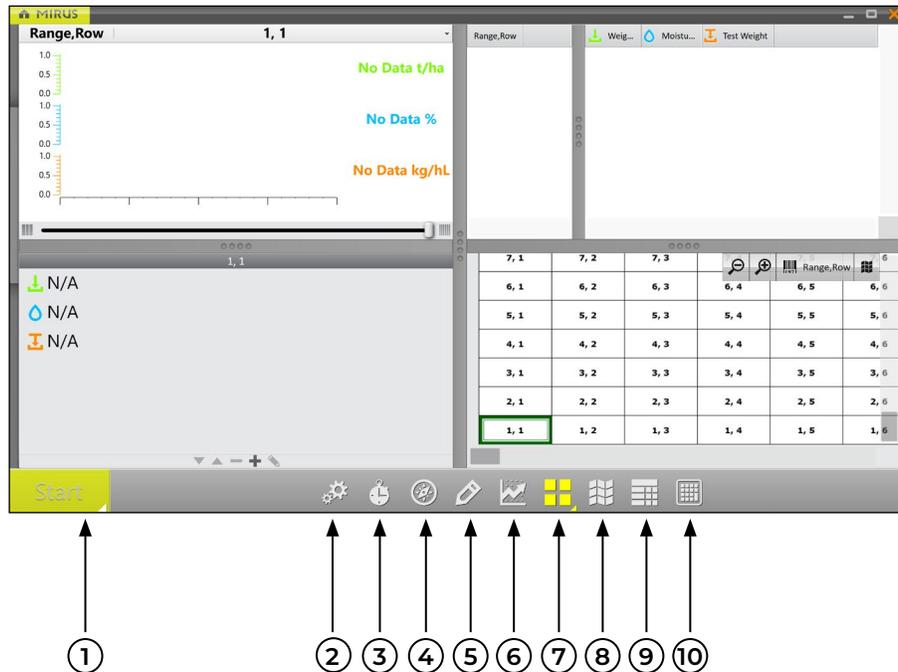
1. **Start/Cycle/Go Button:** **Start** initiates harvest. **Cycle** initiates measurements and data collection for a specific plot. **Go** indicates it's time to move to the next plot.
