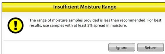
If the moisture content of your samples does not cover a range of at least 3%, Mirus displays an Insufficient Moisture Range warning.
