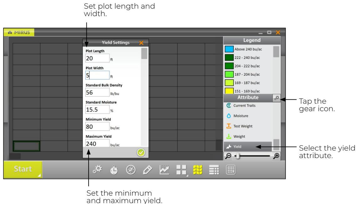
Adjusting the minimum and maximum values helps to create a more detailed legend and define the scope of the graphs and maps. The narrower the minimum and maximum range, the more detailed the information displayed becomes.
