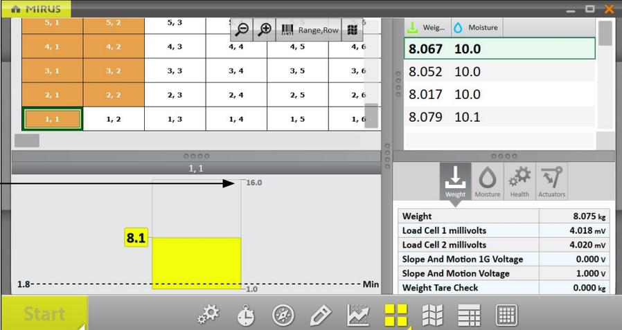
Maximum weight is adjusted on the Real Time Weight display.
