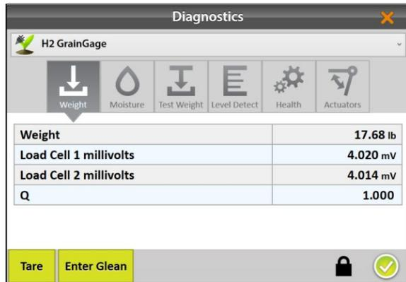
1. After calibrating the weigh bucket, tap the gear icon
