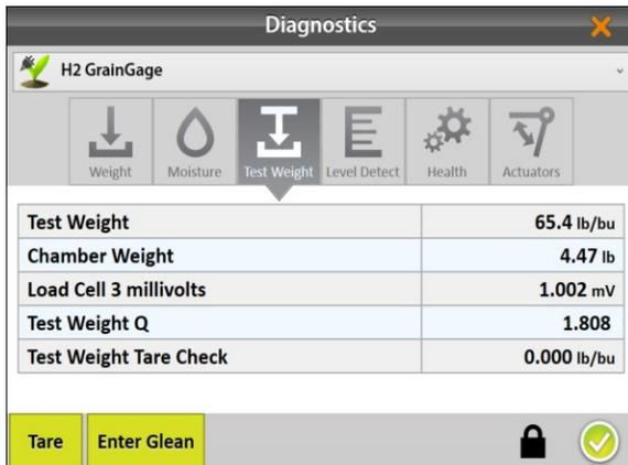
1. After calibrating the test chamber, tap the gear icon
