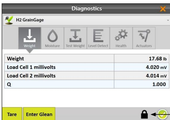
On the Weight Diagnostics screen, live values are shown for the load cells.
