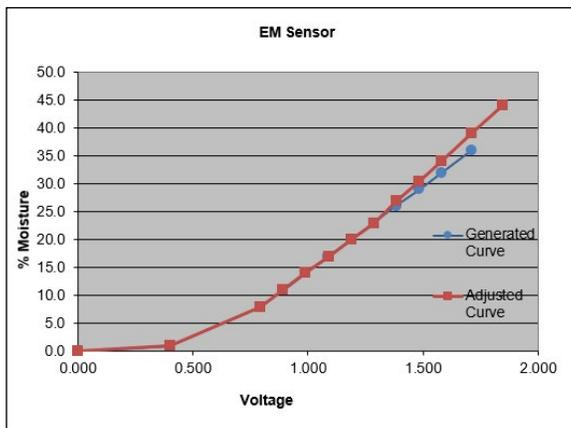
In some cases, the higher the moisture, the steeper the slope of the curve. This is indicated by a *steady increase in the difference* between the moisture curve and the moisture percentages in the grain samples as the moisture values increase.
