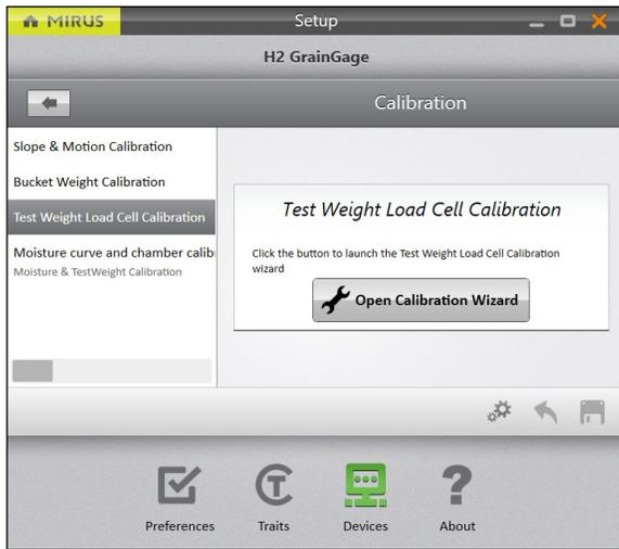
6. Tap **Test Weight Load Cell Calibration**.
