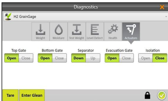
Use the Actuators Diagnostics screen to manually test the actuators controlling all gates connected to the GrainGage. For more information about actuators see **2.3.2 Configure Actuators** on page 17.
