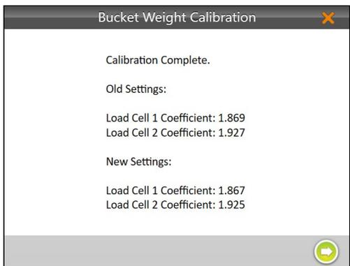
18. Mirus displays the old and new load cell coefficients.
