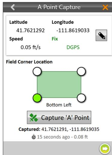
**Step 3:** Establish a bearing by either entering a bearing, if it is known, or by moving several plots through the field to capture the B point. The accuracy of the bearing tends to be better when there is a long distance between the A point and the B point. If these points are captured at a short distance, the bearing could have some error in it
