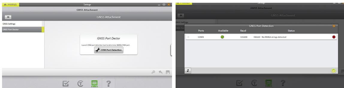
**Step 5:** Select the port that is detected by the software, and go to GNSS settings and set the correct COM port. The following settings are automatically filled in, except for offsets:
