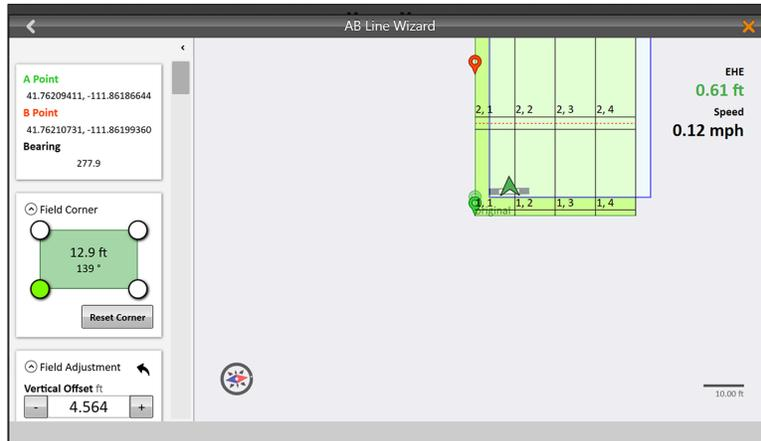
**Step 6:** In the Setup Wizard you can make changes or adjustments to field placement and plot/alley dimensions. Once the layout of the map is set up as desired, select the green check mark to close out of the AB Line Wizard.
