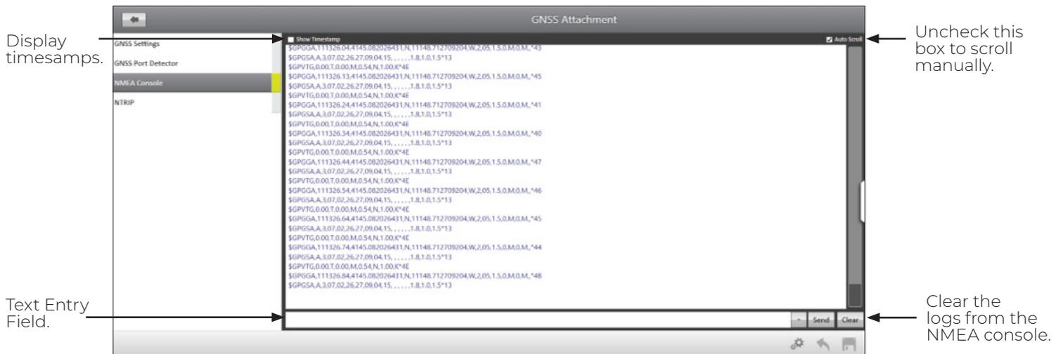
Use the text entry field to send commands or messages to the GNSS receiver. For a comprehensive list of commands and messages that can be used to configure your GNSS receiver, please refer to the technical documentation provided by the manufacturer of the receiver.
