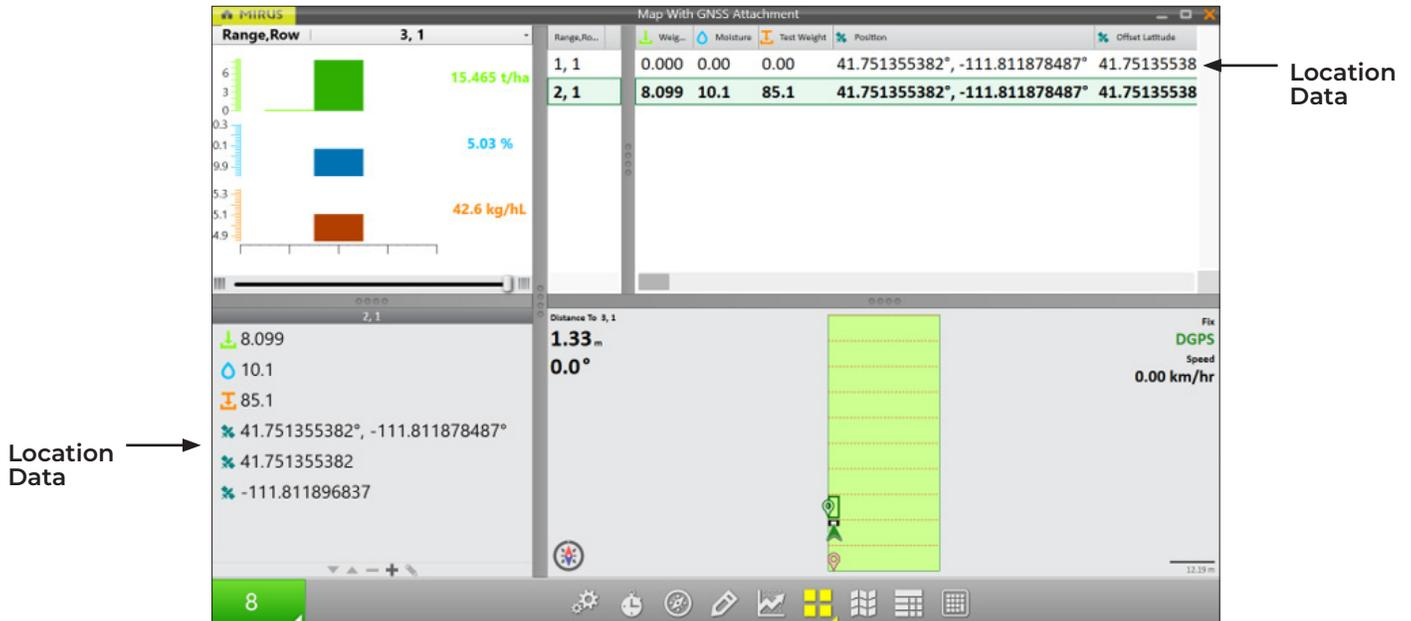
When harvesting, ensure the GrainGage has completed cycling before you arrive at the next trip point. If you drive too fast, you will lose some GNSS data points on the trip. To approximate how fast you are driving, divide the Trip Distance by the cycle time (the time between the isolation door closing and opening) of the GrainGage.
