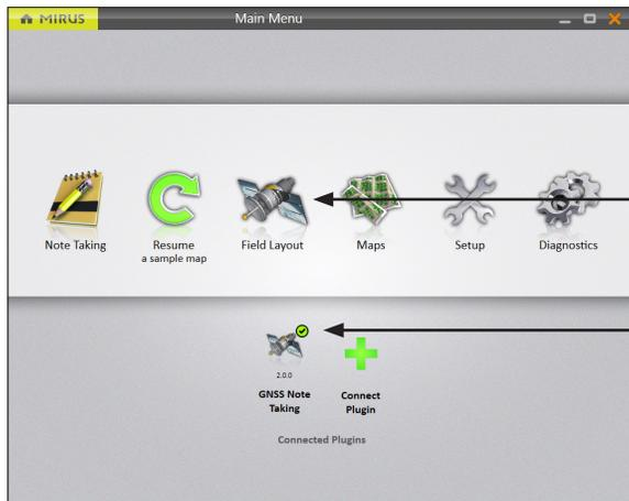
6. Return to the Main Menu. GNSS Note Taking is displayed with a green check mark and Field Layout is added to the menu items.
