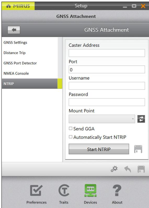
If you have a subscription with an NTRIP service, use the NTRIP screen to enter the address, port, and credentials necessary to connect to the NTRIP caster. On the **Setup > GNSS Attachment/GNSS Note Taking** screen,
