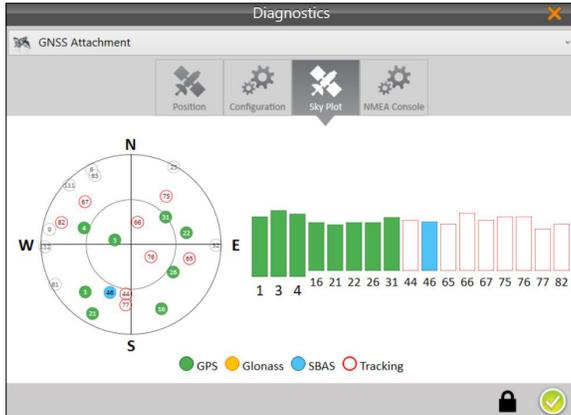
The Sky Plot Diagnostics screen shows the satellites used in the positioning solution and where they are in the sky.
