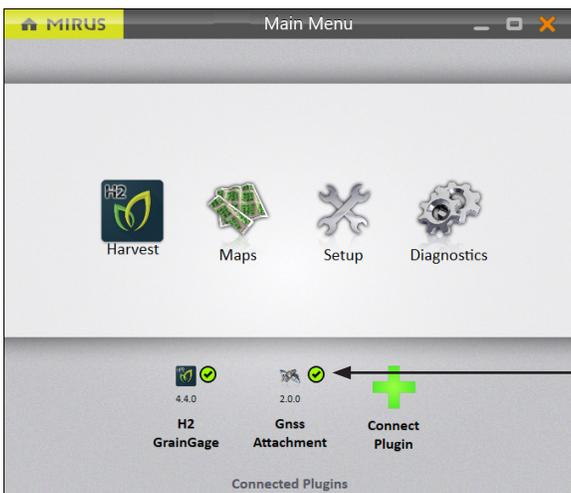
7. Return to the Main Menu. The GNSS Attachment is displayed with a green check mark.
