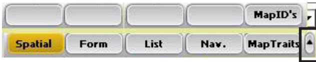
Figure 8-4: Tapping on the up arrow makes the MapID's soft key appear and disappear
