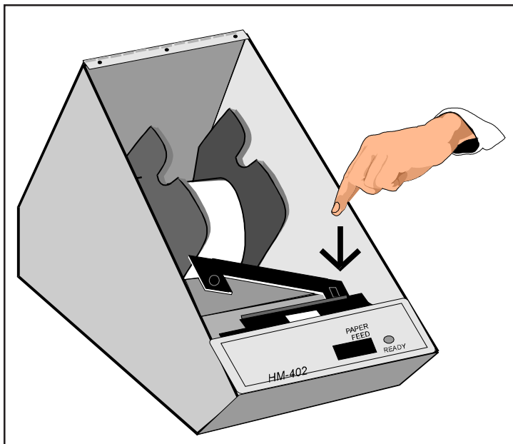
Figure 2-16: Ribbon placement in the HarvestData System FieldPrinter. To remove a used ribbon, press down on the right side of the cartridge (as shown by the arrow) and lift it out. Put a new ribbon in its place.
