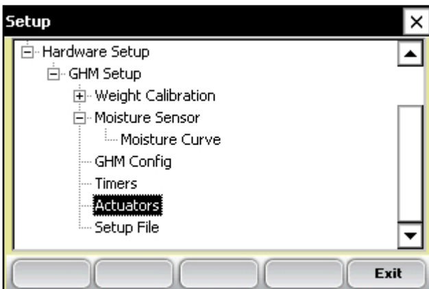
Figure 3-23: Double-tap Actuators from the Setup menu to access the Actuator Setup screen
