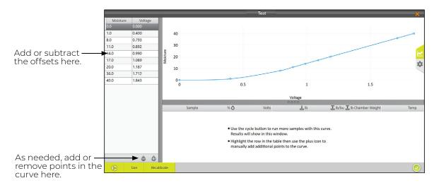
In the example above, readings from the benchtop sensor indicate that the samples have, on average, 1% higher moisture than the percentages in the previously calculated moisture curve.
