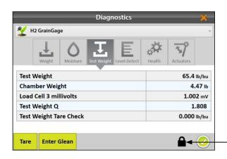
On the Test Weight Diagnostics screen, live values are shown for chamber weight and calculated test weight.
