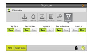
Use the Actuators Diagnostics screen to manually test the actuators controlling all gates connected to the GrainGage. For more information about actuators see **2.3.2 Configure Actuators** on page 17.
