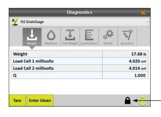
On the Weight Diagnostics screen, live values are shown for the load cells.
