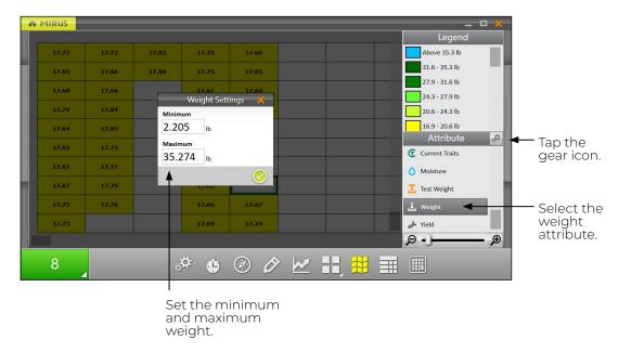
This setting adjusts the maximum weight on the Real Time Weight display, which allows you to track how full the GrainGage is getting with each plot. This is important to monitor so the GrainGage doesn't overflow.
