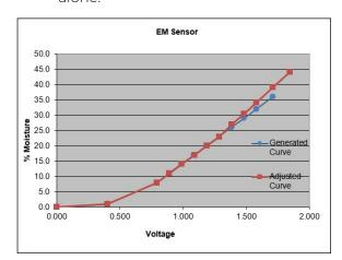
In some cases, the higher the moisture, the steeper the slope of the curve. This is indicated by a *steady increase in the difference* between the moisture curve and the moisture percentages in the grain samples as the moisture values increase.
