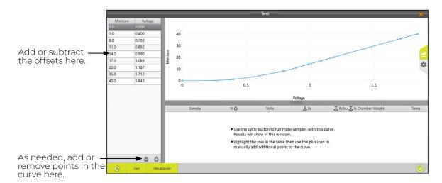
In the example above, readings from the benchtop sensor indicate that the grain samples above 26% have, on average, 1% higher moisture than the percentages in the base moisture curve. Therefore, in the curve:
