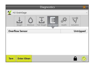
On the Level Detect Diagnostics screen, Mirus displays the status of the Level Detect Sensor. It should be Untripped when the weigh bucket is empty.
