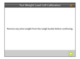
13. Check for and remove any extra weight from the weigh bucket.
